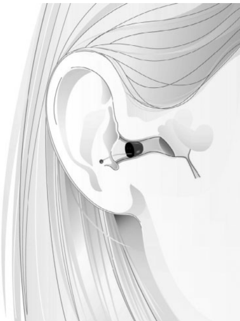
FIGURE 38.5 An invisible-in-the-canal [IIC] hearing aid. [Courtesy of ReSound.]
