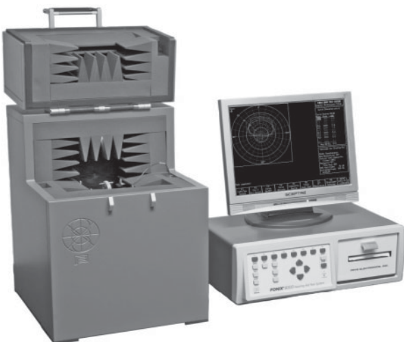
FIGURE 38.13 Two examples of hearing aid test boxes. [Courtesy of Audioscan ( top ) and Frye Electronics ( bottom ).]
