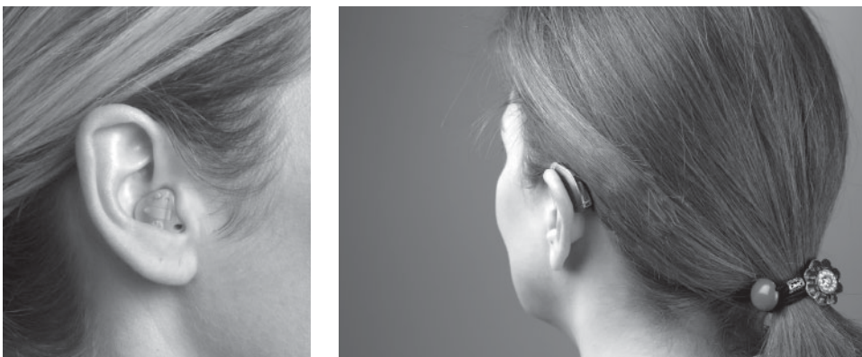
FIGURE 38.1 An example of an in-the-ear [ITE] and a behind-the-ear [BTE] hearing aid as worn by a hearing aid user. [Courtesy of ReSound [left] and Starkey Laboratories [right].]
