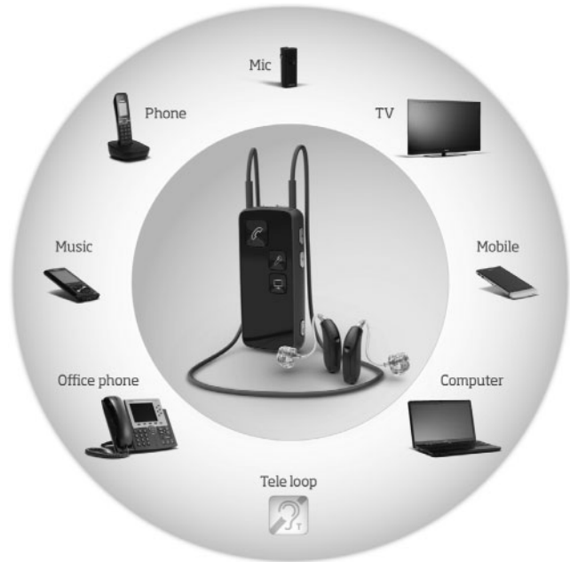
FIGURE 38.23 An NFMI digital wireless hearing instrument system. [Courtesy of Oticon.]
