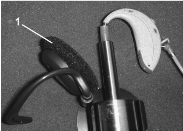
FIGURE 39.15 Setup for inducing controlled feedback in the test chamber. The monitor headphone [1], which is normally used to listen to the output of the hearing aid in the coupler, is placed near the hearing aid. The monitor gain is adjusted to induce feedback.
