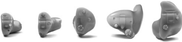
FIGURE 38.4 Examples of ITE hearing aids. [Courtesy of ReSound.]
