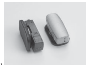
FIGURE 43.1 Photos of the Baha, Ponto, and Sophono bone-conduction hearing aids.
