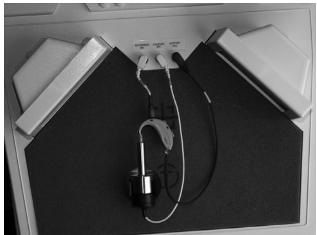
FIGURE 38.14 Configuration of the hearing aid, coupler, and microphone for hearing aid testing. [Courtesy of Audioscan.]
